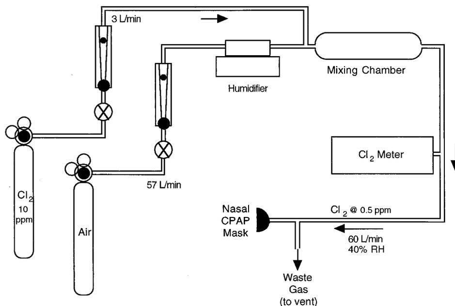
**FIG 2.** Schematic of chlorine dilution apparatus. Note that exposure was by nasal mask with scavenger hose attached to T-piece, allowing subject to transition from exposure to physiologic testing without leaving climate-controlled chamber. CPAP, Continuous positive airway pressure.
